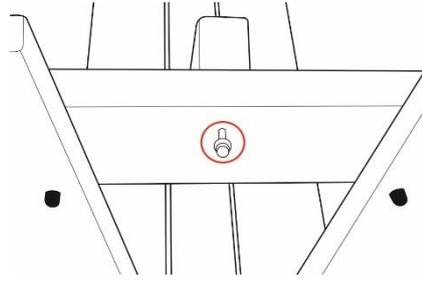
Ensure that the brace is lined up centrally on the bench and attach it to the A-frame with a coach screw
