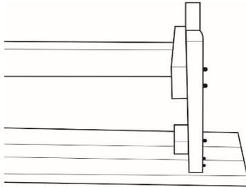
For a 3ft or 4ft set, take one of the bench braces (rectangular) and align it between the two A-frames
