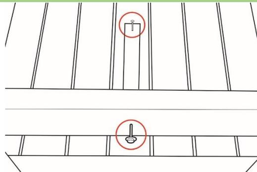
Ensure that the brace is lined up centrally on the table and attach it to the A-frame with a coach screw
