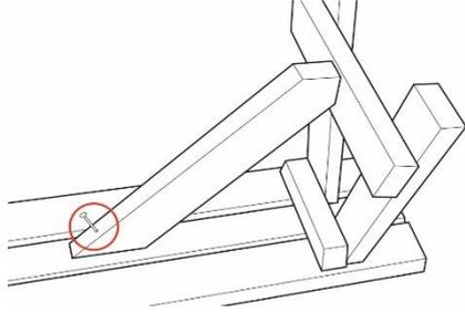
For a 5ft to 8ft set, place a shorter brace aligned centrally on the seat as shown and affix to the bench with a coach screw
