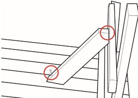
Place a longer cross brace in position as shown, ensuring that it is flush with the underside of the table A-frame and proceed to step 4
