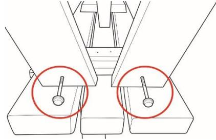
Place one of the bench A-frames centrally against the fixing batten ensuring that the gap at the bench edge is the same on both sides. Now, using 2 of the supplied coach screws and the predrilled holes, secure the bench A-frame to the fixing batten on the seat and repeat for the remaining 3 A-frames.
