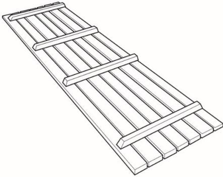
Lay the tabletop upside down on a clean, flat surface taking care not to damage it. Now line up one of the table A-frames centrally on the tabletop as shown in step 2
