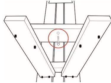
Secure into place using 2 coach screws at either end as shown
