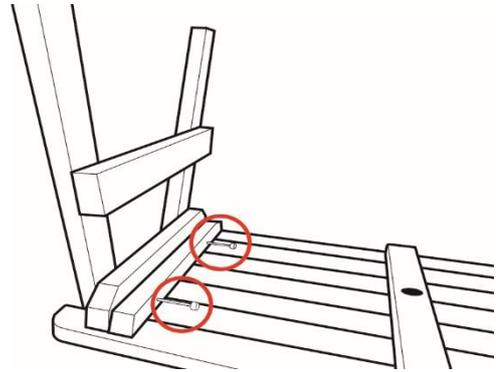
Place one of the table A-frames centrally against the fixing batten ensuring that the gap at the table edge is the same on both sides. Now, using 2 of the supplied coach screws and the predrilled holes, secure the table A-frame to the fixing batten on the tabletop.
