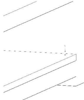
Ensure the shelf is lined up with the front of the leg and secure into place with the 40mm screws supplied, use predrilled guide holes.
