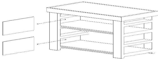
For double shelf version, fit the side panels into position. Centralize and secure with 40mm screws using pre-drilled guide holes.
