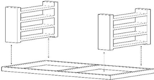
Lay the top upside down and place a leg in position as shown. Ensure the leg is pushed into the corner and secure with the supplied 60mm screws use pre-drilled guide holes.
