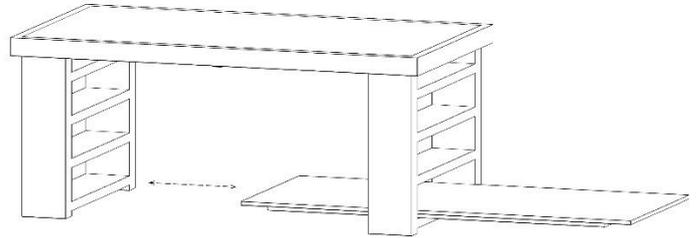
Fit the bottom shelf into position. Keep the shelf straight, parallel to the table.
