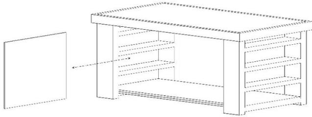
Fit the side panels in position. Centralize and secure with 40mm screws using pre-drilled guide holes.
