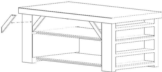
Ensure the brace is pushed flush with tabletop and leg frame and secure into place, repeat this step on the other leg.
