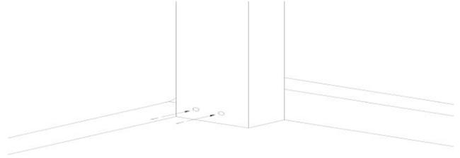
Ensure the leg is pushed into the corner and secure with the supplied screws.
