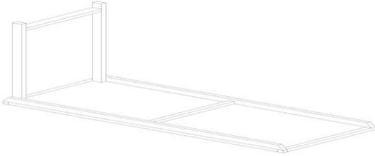
Lay the top upside down and place a leg in position as shown.
