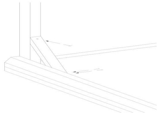
Ensure the brace is pushed flush with tabletop and leg frame and secure into place.
