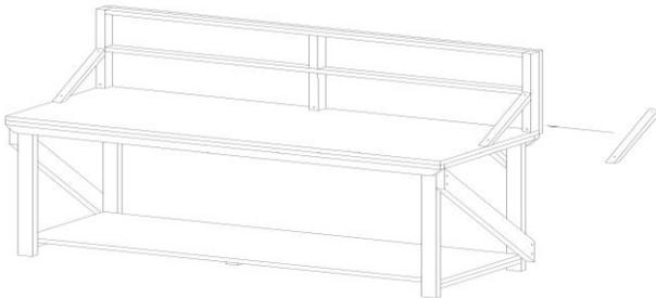
Fit the side brace and secure using the supplied screws.
