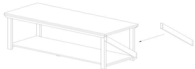
Add side braces, ensure the brace is pushed into the top corner and is lined up with the front of the leg and secure into place.
