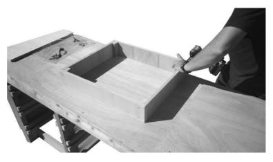
Secure sides with goldens screws using pre-drilled guide holes. Make sure that all panels are flush with each other.
