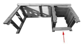
Place front-bottom panel away you to have cupboard on left hand side and secure with provided screws.
