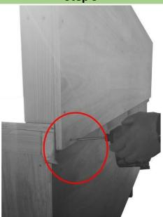
If you chose workbench with back panel, please put into place as shown in the picture and secure it with golden screws from the back.
