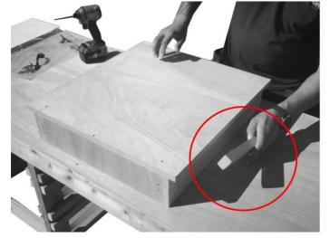
Put base as shown in the picture and use two provided battens from each side to get correct distance from each end and secure with provided screws.
