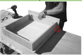
Place drawer front panel and make sure it is even spaced out on both sides. Secure with provided screws. **Repeat steps 1 to 1.4 to complete rest of the drawers.**
