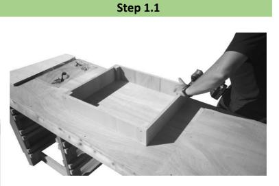
Secure sides with goldens screws using pre-drilled guide holes. Make sure that all panels are flush with each other.
