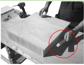
Put base as shown in the picture and use two provided battens from each side to get correct distance from each end and secure with provided screws.
