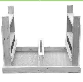
Place middle brace and last leg into position. Ensure that middle brace is as shown in the picture. Also push all parts flush with tabletop support and secure into position as shown in the step 1.2 (3ft version workbench do not have middle brace)
