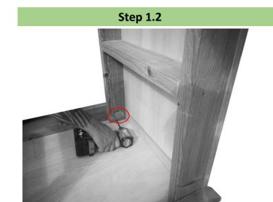
Secure with the supplied screws use pre-drilled guide holes.
