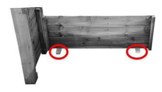
Stand the left-hand end panel upright on a flat, level surface. Arrange two spacer blocks on the ground, adjacent to the panel.
