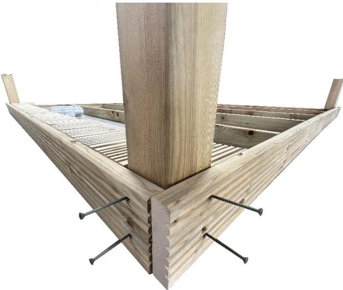
When all your decking boards are secured, arrange the upstand edge decking pieces around the base's perimeter, ensuring the edges are aligned. **Important:** push/pull the upstand up or down, if necessary, before fixing it into place with shorter wood screws. Continue to step 12 for the pergola assembly.
