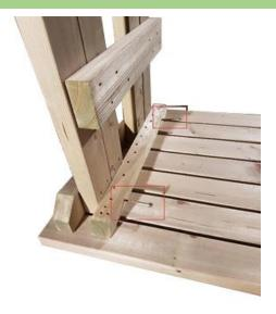
Now, using 2 of the supplied coach screws and the pre-drilled holes, secure the table frame to the fixing batten on the tabletop.
