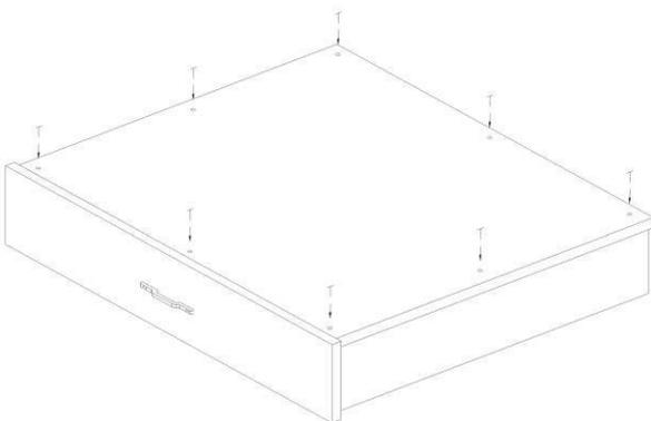
Finally, secure base with golden screws using pre-drilled guide holes
