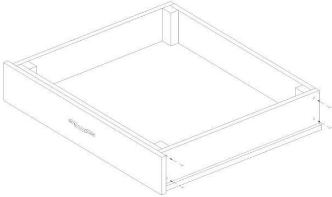
Secure sides with golden screws using pre-drilled guide holes. Make sure that all panels are flush with each other.
