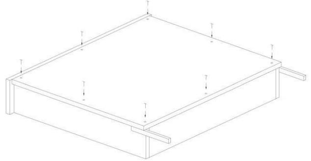
Put base as shown in the picture and use two provided battens from each side to get correct distance from each end.
