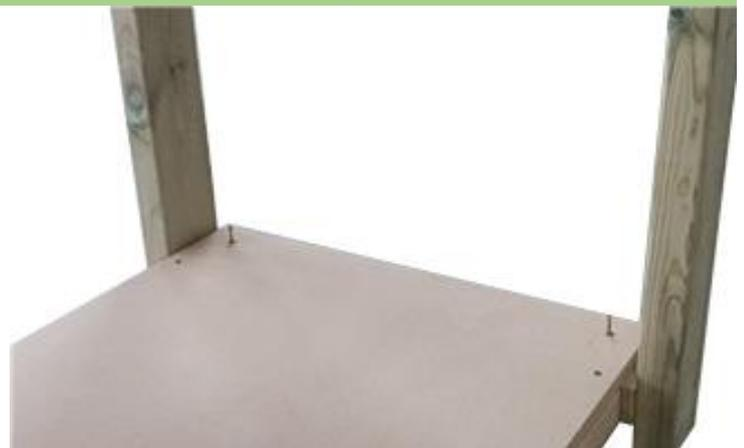
Place table back on its feet. Slide the bottom shelve into position. Keep the shelve straight, parallel to the table, centralize and secure with provided golden screws.
