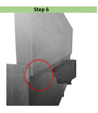
If you chose workbench with back panel, please put into place as shown in the picture and secure it with golden screws from the back.
