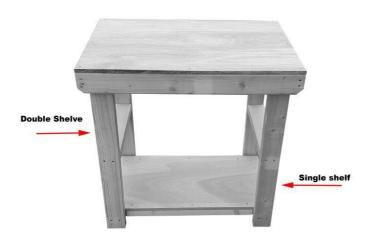
Now, place braces as shown in the picture and secure using 60mm screws via pre-drilled guide holes. Make sure that braces are flush with leg upright and tabletop. **Repeat**this step on both sides.
