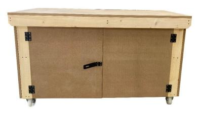
Place the door vertically and horizontally for a good fit and secure the doors to the legs, as shown in the picture.
