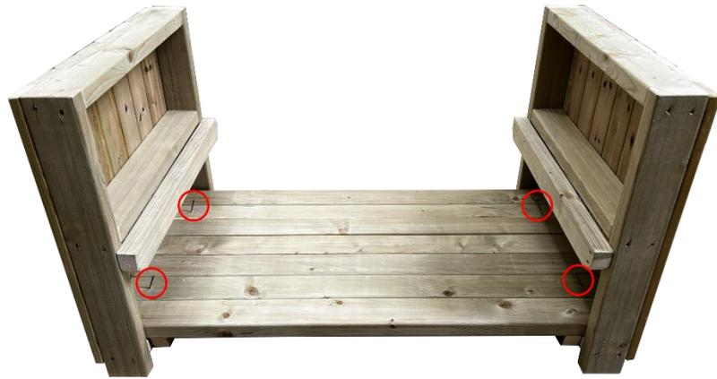
Stand both of the table legs parallel straight from one to another, fit the shelf to the lower leg position, make sure that the shelf is pushed to one of the corners, leaving a gap on the other side for the back panel attachment, and secure it using 4x 60mm wood screws.
