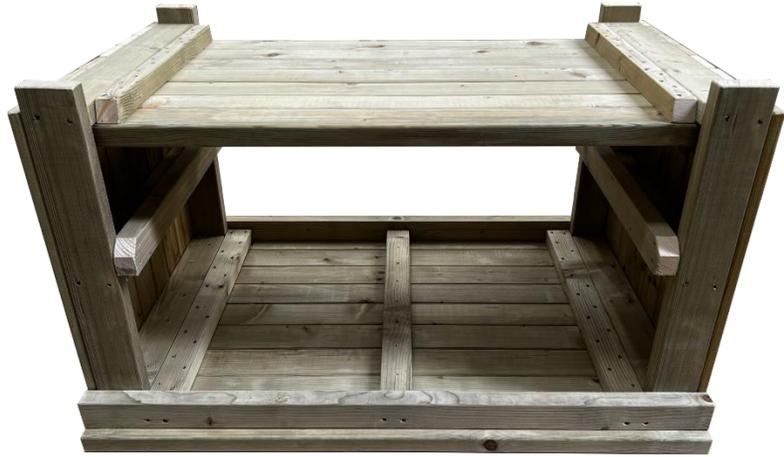
Now, place the worktop on a flat and even surface, making sure that the tabletop is facing the ground. Carefully flip your current assembly upside down and gently position it on the tabletop, making sure that all the edges are aligned.
