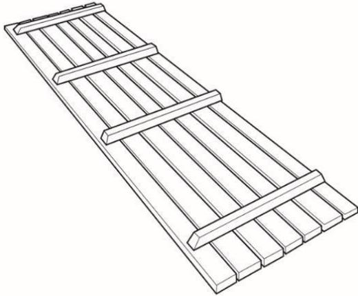
Lay the tabletop upside down on a clean, flat surface taking care not to damage it. Now line up one of the table A-frames centrally on the tabletop as shown in step 2
