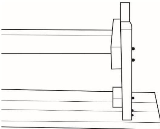
For a 3ft or 4ft set, take one of the bench braces (rectangular) and align it between the two A-frames
