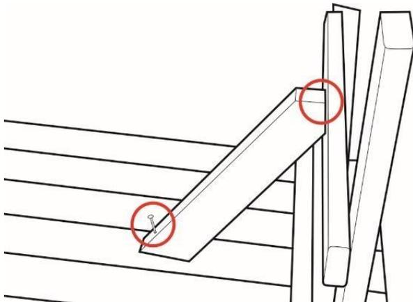
Place a longer cross brace in position as shown, ensuring that it is flush with the underside of the table A-frame it to the A-frame with a coach screw and proceed to step 4
