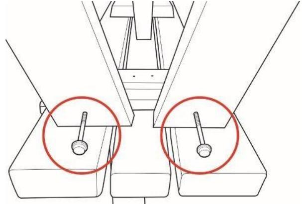
Place one of the bench A-frames centrally against the fixing batten ensuring that the gap at the bench edge is the same on both sides. Now, using 2 of the supplied coach screws and the predrilled holes, secure the bench A-frame to the fixing batten on the seat and repeat for the remaining 3 A-frames.
