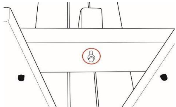
Ensure that the brace is lined up centrally on the bench and attach it to the A-frame with a coach screw.
