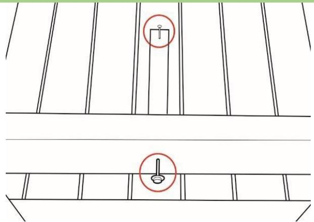
Ensure that the brace is lined up centrally on the table and attach
