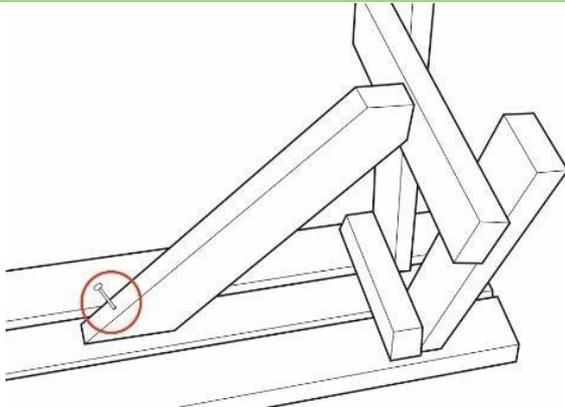
For a 5ft to 8ft set, place a shorter brace aligned centrally on the seat as shown and affix to the bench with a coach screw.
