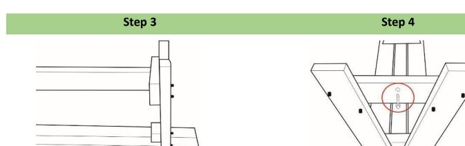
For a 3ft or 4ft set, take one of the bench braces (rectangular) and align it between the two A-frames.
