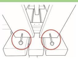
Place one of the bench A-frames centrally against the fixing batten ensuring that the gap at the bench edge is the same on both sides. Now, using 2 of the supplied coach screws and the predrilled holes, secure the bench A-frame to the fixing batten on the seat and repeat same move on the other side.
