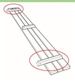
Lay one of the bench seats face down on the flat surface as you did with the tabletop. **Make sure that** you are using benchtop with extended braces.
