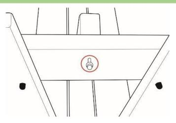
Ensure that the brace is lined up centrally on the bench and attach it to the A-frame with a coach screw.
