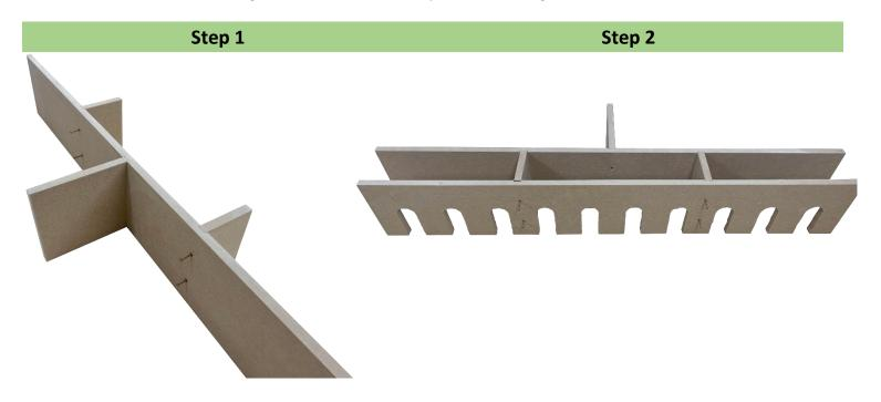
For Step 1 of the assembly process, begin by taking one of the middle panels. Then, attach three of the section dividers to the routed area by securing each one with two of the provided wood screws. In Step 2, you'll need to take the tool holder panel and add it to the two-section divider panels that you previously secured in place. Use four of the provided wood screws to ensure a secure attachment.
