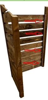
Using the 65mm screws provided, attach the batten on the back panel to the post of the end panel, ensuring that the batten remains vertically aligned to the post. Align one of the longer posts **(shorter for a reversed roof)** with the other end of the back panel. And secure it with the provided screws. Repeat steps 1-4 to complete the rest of the triple log store bays.
