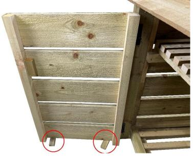
Place a spacer block at the front of the log store adjacent to the front-end post and rest the hinge side of the appropriate door on the block, aligning it vertically and horizontally for a good fit. Now use four of the supplied black hinge screws to affix the hinge to the post.
