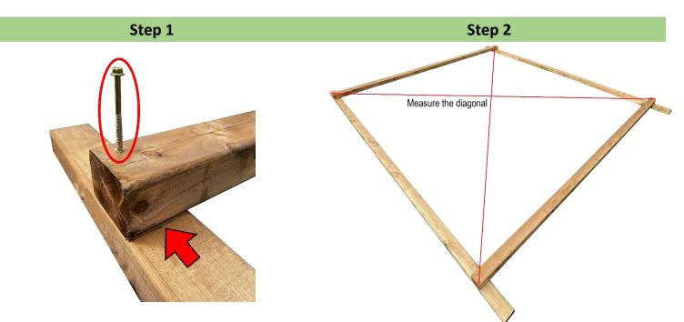
Take two of the smaller slides and place them on two of the longer slides as shown in the picture, before securing it with the coach screw or the metal corner make sure that the shorter slides are properly aligned with the marked line.
