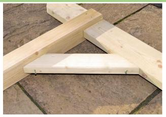
Secure via provided guidelines with wood screws, repeat for the other side as well.
