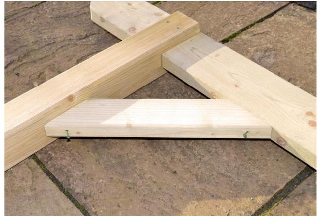
Secure via provided guidelines with wood screws, repeat for the other side as well.
