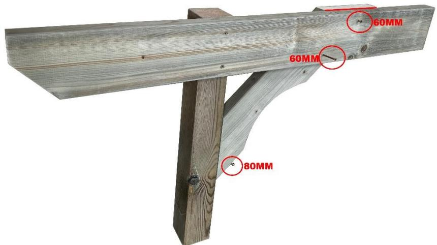
Secure the runner to the post with the 80mm screws.
