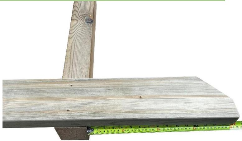
Take one of the posts and one of the runners and arrange on the floor as shown. Align the post to the marked pencil lines on the runner.
