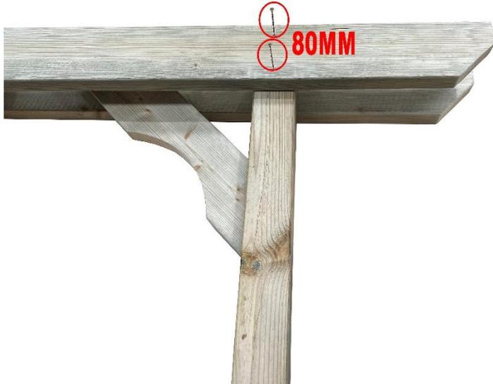
Rotate your assembly and place the second runner in the same manner as the first one aligning both runners and leaving the overhang of 41cm. Secure it with 80mm screws.
