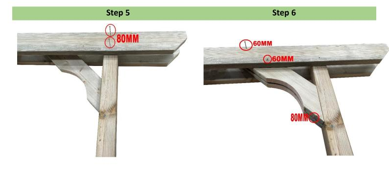
Rotate your assembly and place the second runner in the same manner as the first one aligning both runners and leaving the overhang of 41cm. Secure it with 80mm screws. Take the second brace and attach it in the same manner as the first one making sure that it is properly aligned. If you bought a pergola with rafters, please continue to step 7.
