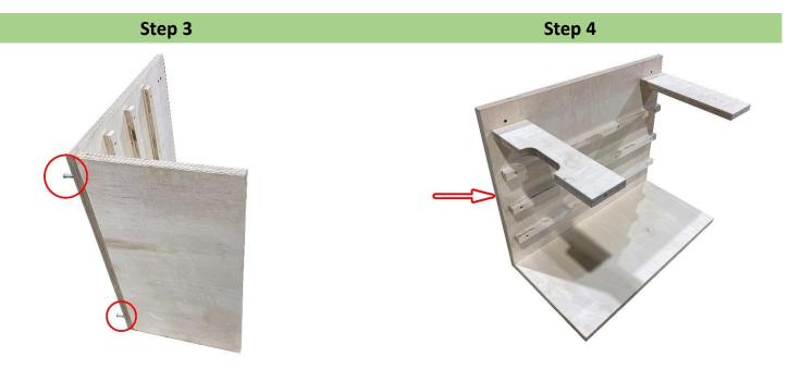
Take the panel from the step 2 and attach the second panel which is shown in the picture with the confirmat screws.
