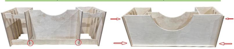
Take the panel which is shown in the picture and secure it with the confirmat screws
