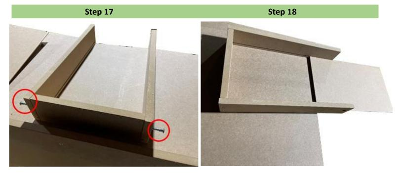
Attach the drawers back panel that the cut out for the board would be facing the same direction. And now secure it with the confirmat screws.
