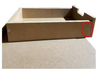
Now place the drawers front panel and secure it with the cam locks from each side. Repeat steps 16 to 19 to finish assembling the rest of the drawers.
