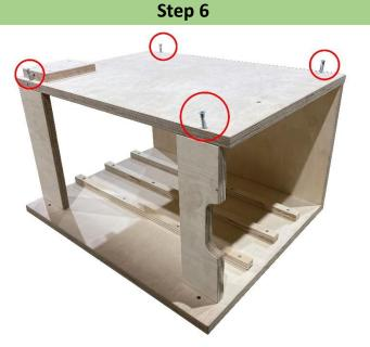
Place the panel which is shown in the picture on your assembly and secure it with the confirmat screws. \*Please note that the front of your assembly must have some free space just as shown in the picture. \*
