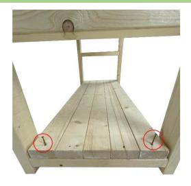
Fit the bottom shelf in position. Centralize and secure using the screws supplied.
