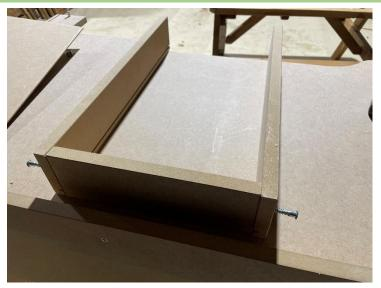
Attach the drawers back panel that the cut out for the board would be facing the same direction. And now secure it with the confirmat screws.
