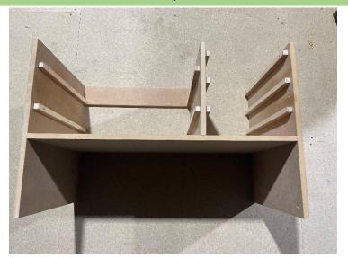
After ensuring the side panels, attach one of the support panels just as shown in the picture and secure it with the provided confirmat screws.
