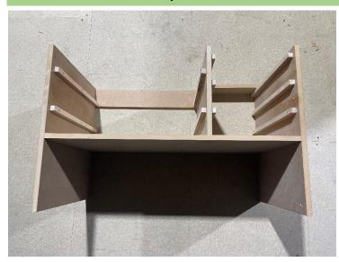
Take another provided support panel and place it just as shown in the picture, securing it with the confirmat screws. Step 6
