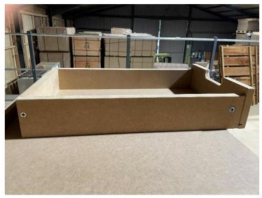
Now place the drawers front panel and secure it with the cam locks from each side. Repeat steps 15 to 15.3 to finish assembling the drawers.
