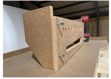
Assemble tool holder panel parts just as shown in the picture and secure it with the confirmat screws.
