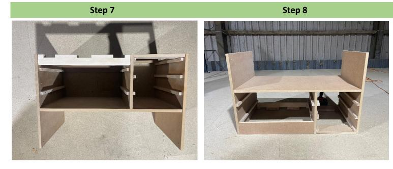
Place the routed plank in the position shown in the picture and ensure it with the confirmat screws.
