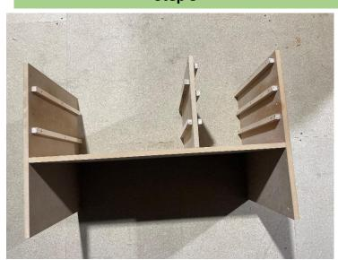
Now take 2x of the side panels and place just as shown in the picture that the rails would match each other. Ensure it with the confirmat screws.
