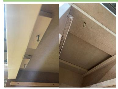
Underneath the workbench, you will find 3x holes which need to be secured with the provided screws.
