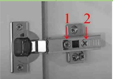
Start first by adjusting machine screw market as number one on the arm of the hinge, this will adjust your door left-to-right or horizontal position. If you need to adjust in and out position simple adjust cam-screw marked as number two. To adjust up and down or vertical position, simple release hinge plate.
