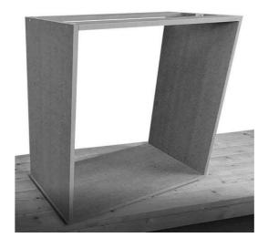
Take both partitions (AGS4\_2) align with pre-drilled guide holes and secure with provided confirmat screws.
