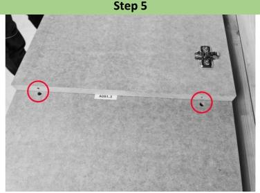
Take base panel (AGS4\_3) and align with side panel (AGS4\_1) pre-drilled guide holes as shown in step 5.
