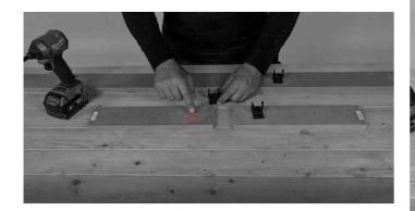
Last step is to cover legs with a panel. Take leg panels (AGS\_2) and secure leg supports using pre-drilled guiles and wood screws.
