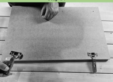
Now take your doors (2x AGS3\_5). Place hinges into pre-drilled holes and secure with wood screws 4x16mm. Repeat this step for all three doors.
