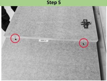
Take base panel (AGS3\_3) and align with side panel (AGS3\_1) pre-drilled guide holes as shown in step 5.
