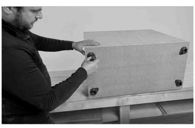
At this stage, take 4 cabinet legs and secure them into place as shown in the picture. These legs are adjustable heigh 100mm to 130mm. You can adjust them at this stage or later when you will position your cabinet into upright position.
