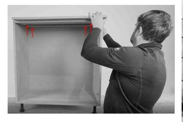
Filp your finished construction to upright position. Take your tabletop (AGS3\_7) and secure via pre-drilled guide holes as shone in the picture.
