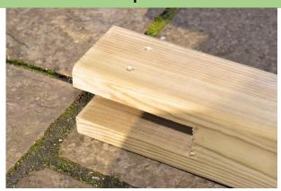
Lay down one of the posts with the slot parallel to the ground as shown.
