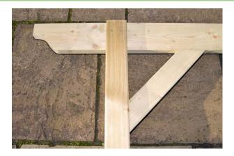
Place one of the diagonal braces (500mm) in place, adjusting the post angle if necessary, so that it butts snugly up to the inner edge of the runner and post. This ensures that it is set at 90°.
