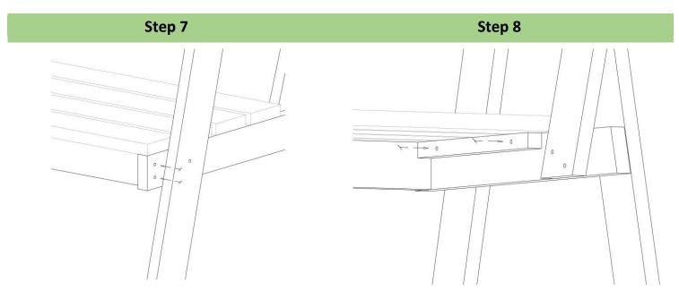
Align the seat panel flush with the front edge of the end screws frame as shown and secure in place using 2x 85mm repeat for screws. Repeat for the other leg frame. Working from underneath the seat panel use 2 coach to attach the seat panel to the leg frame and then the other side.
