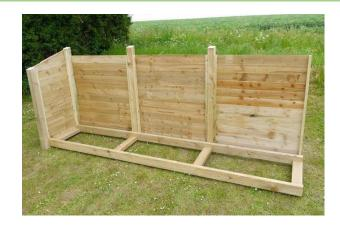
Remove the blocks from beneath the 3rd panel and then slide the base into position as shown.
