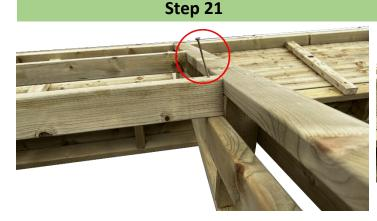
Add the roof rafters to the shelter, ensuring alignment with the triangle dividers. Secure each end of the roof rafter using the provided 120mm wood screws.
