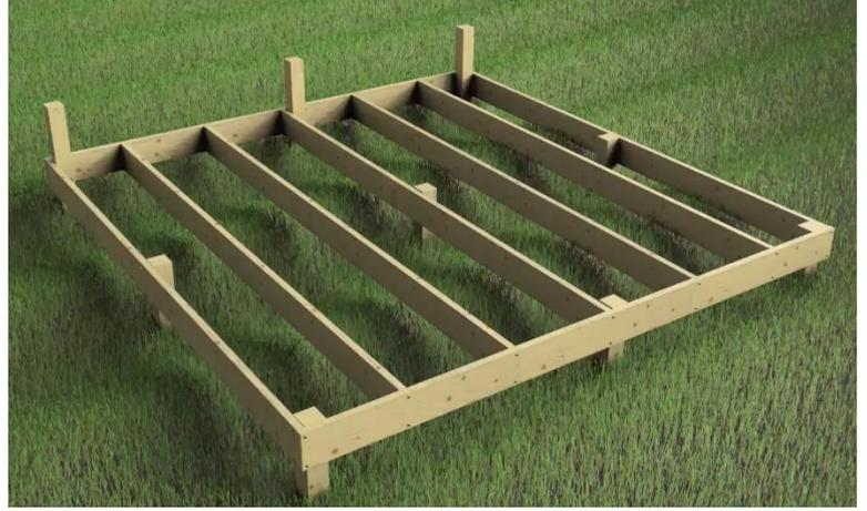
Or used as supports on uneven ground, with the use of slabs to prevent subsidence if necessary. **Important! On both options, the use of a spirit level is essential**, To check that the posts and the frame are still vertically and horizontally.
