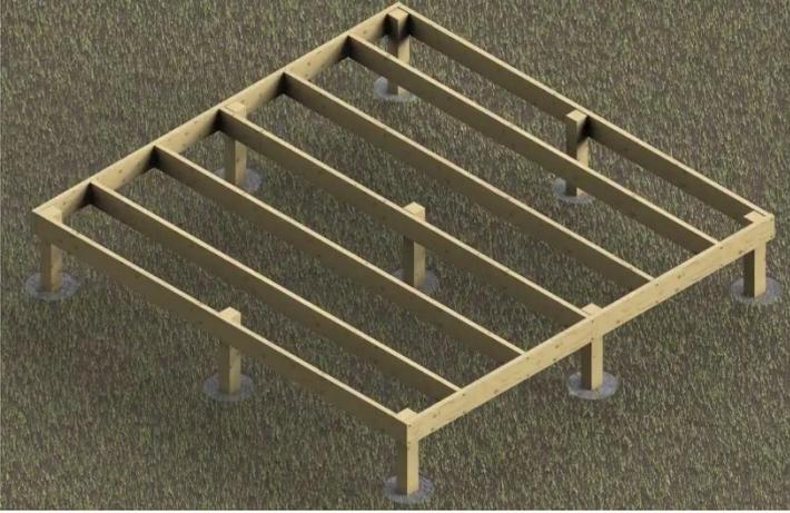
If decking frame supports are used, they can be concreted into the ground as shown.
