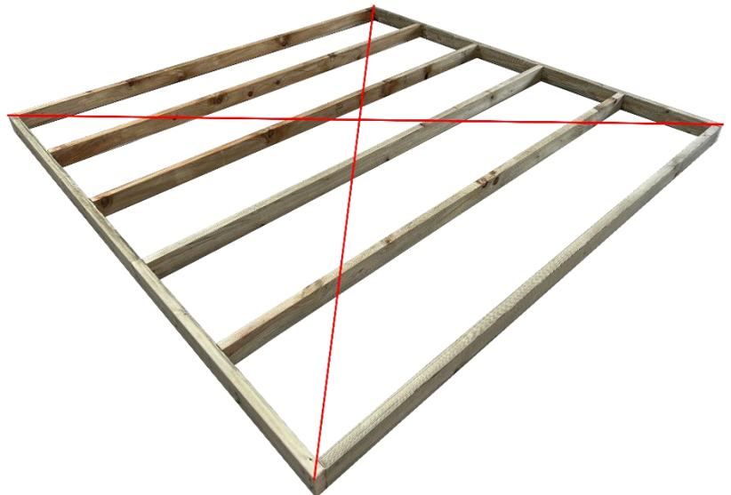
**Important:** After securing each timber plank with wooden screws, measure the diagonal on both ends so that they would be equal.
