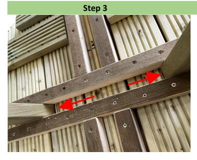
As you place the leg into position, ensure that it aligns perfectly with the marker-marked lines on the tabletop. These lines are specifically provided to help you center the table legs in the middle of the tabletop, ensuring a balanced and aesthetically pleasing appearance.
