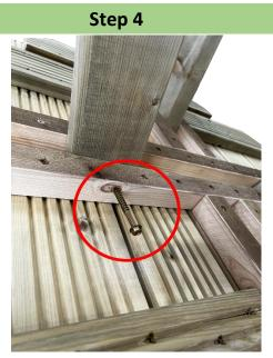
Secure each leg to the tabletop by utilizing the provided coach screws through the predrilled pilot holes. Insert the coach screws carefully into the pilot holes, ensuring they are tightly fastened to establish a strong and stable connection between the legs and the tabletop.
