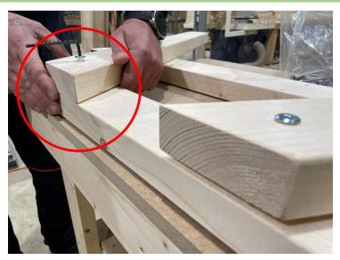
Before securing the top of the leg with bolts and nuts make sure that it is aligned and sits parallel straight with the other side of the leg. After aligning and screwing the top of the A-frame secure the rest of the bolts with the provided nuts.
