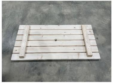
Lay the tabletop upside down on a clean, flat surface taking care not to damage it. Now line up one of the table A-frames centrally on the tabletop as shown in step 6.
