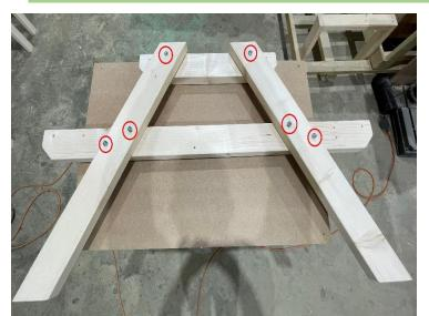
Place 2x planks which are shown in the picture on top of the previous planks making sure bolts fitted previously goes through the correct pilot holes.
