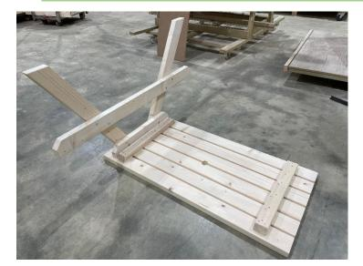
Place one of the table A-frames centrally against the fixing batten ensuring that the gap at the table edge is the same on both sides.
