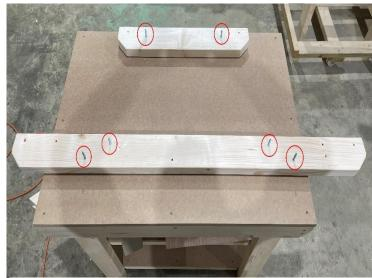
Ensure that you have all of the correct parts as listed on the front page of these instructions, including any fixings. Put the provided bolts in the marked holes to the same planks which are shown in the picture and make sure that the bolt ends are facing up.
