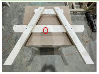
This is how your finished A-frame leg should look like. Repeat steps 2 to 4 to finish the other leg. Before assembling the other leg make sure that the hole which is marked in the picture would be facing the same direction as it is on the first leg.
