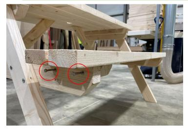
Align the seat panel batten with the outer end of the A-frame as shown and repeat for the other end of the seat panel. Using the coach screws provided attach the seat panel to the A-frame at both ends of the bench.
