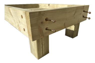
Ensure the main beam is butted against the edge rafter and all the edges are flush. Please note that the main beams have 2x3 batten attached and your pre-drilled pilot holes should be on the outer side. Secure main beams with 100mm coach bolts. Repeat this step for the other side.
