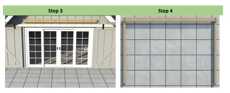
Attach the wall plate using suitable fixings for the wall construction. Measure in 400mm from each end and use 5 fixings distributed evenly and vertically centred across the wall plate secure it to the wall, making sure it is horizontal with a laser or spirit level.
