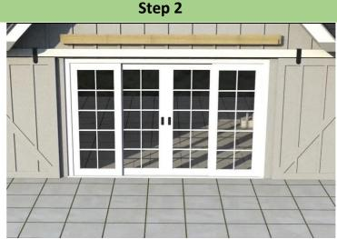
Work out where you wish to affix your wall plate, ensuring that it is positioned so that the area directly in front of it is flat, level and able to support the structure.
