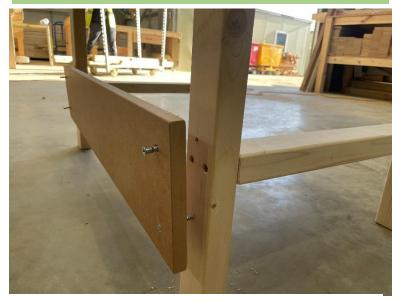
Rotate the workbench on its legs and attach the back panel on the back of the workbench use the pre-drilled pilot holes to secure the back panel with the provided confirmat screws.
