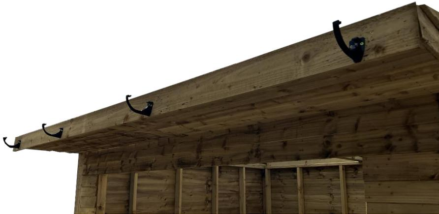
Begin by securing the gutter holders along the front edge of the shelter, leaving approximately 15 cm of space from the edges. Ensure that the gutter holders are not fixed at the same level. For proper water drainage, follow these guidelines:
