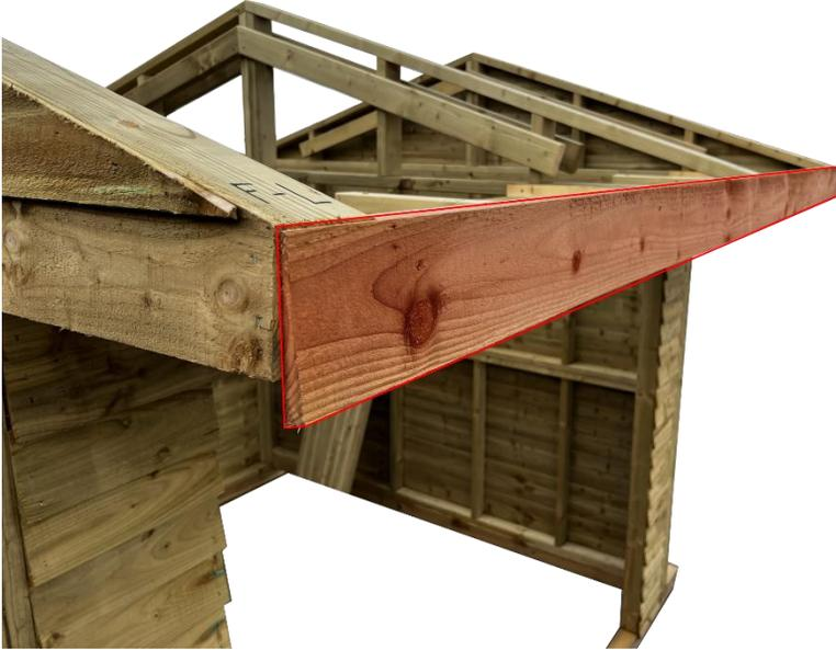
Take the roof front featheredge cover board. Align the pointy end of the cover board with the roof structure, as shown in the illustration or picture. Secure the board in place using 40mm wood screws.
