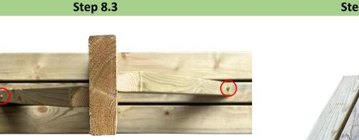
Once the braces are secured to the third leg, attach the other end of each brace to the bench top using the provided coach screws, using the predrilled pilot holes.
