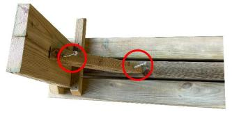
Place a seat leg brace in position and, as you did for the table. Ensure it is centrally aligned. Attach one of the seat leg braces to the other end of the seat unit and then repeat until both seats are done. If you have an 8ft version than please continue to step 8.1 if not you can skip to step 9.
