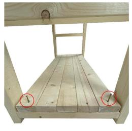
Fit the bottom shelf in position. Centralize and secure using the screws supplied.
