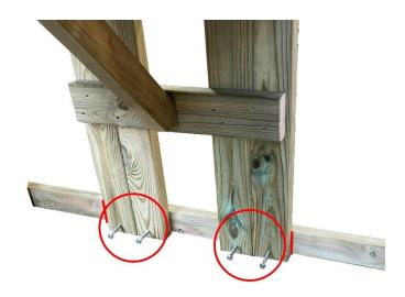
Turn the table right side up. Place one of the leg braces centrally against the table leg frame as shown.
