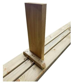
Measure the distance between the left and middle battens and then between the middle and right battens on the underside of the bench top, and place the third middle support leg, made from a 2x6 timber plank, in the middle of the larger gap, securing it with two of the provided coach screws.
