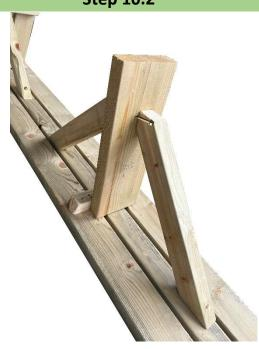
Take two of the support braces, align them with the predrilled holes on the third support leg, and secure them to the middle leg using the provided screws.
