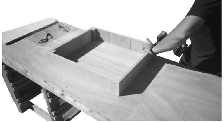
Secure sides with golden screws using pre-drilled guide holes. Make sure that all panels are flush with each other.
