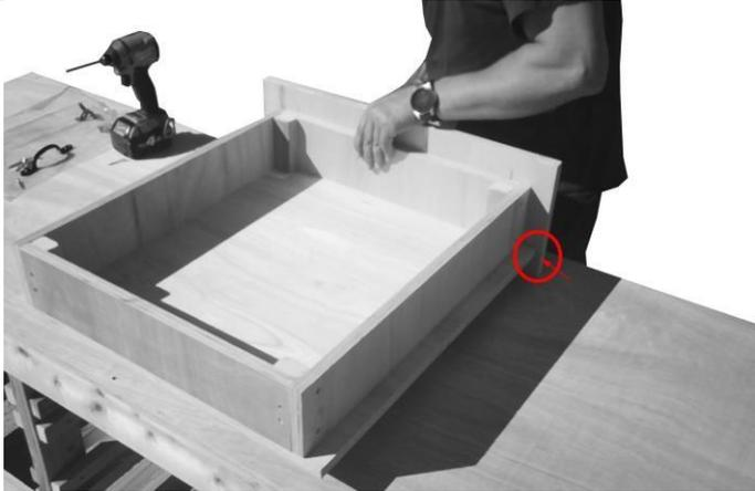
Place drawer front panel and make sure it is even spaced out on both sides. Secure with provided screws. **Repeat steps 1 to 1.4 to complete rest of the drawers.**
