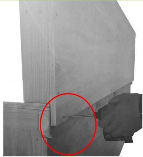
If you have workbench with back panel, please put into place as shown in the picture and secure it with golden screws from the back.
