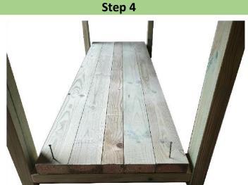
Ensure the brace is pushed flush with tabletop and leg frame and secure into place, repeat this step on the other leg.
