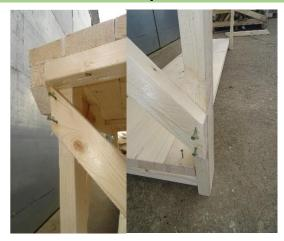
Ensure the long brace is pushed flush with tabletop and leg frame and secure into place, repeat this step on the other leg.
