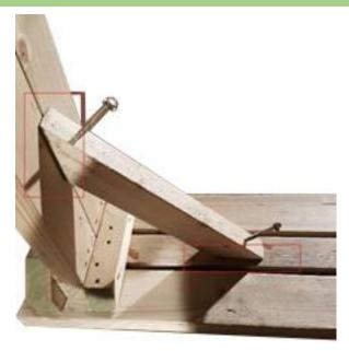
Place a cross brace in position, ensure that it is flush with the underside of the bench frame.
