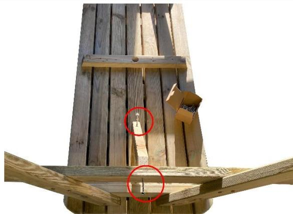
Ensure that the brace is lined up centrally on the table and attach it to the A-frame with a coach screw. Make sure that the brace is still aligned centrally on the table and affix the other end to the tabletop with a coach screw as shown. Repeat steps 1-4 to finish the table assembly and proceed to step 5.
