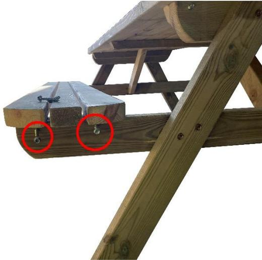
Align the seat panel batten with the outer end of the A-frame as shown and repeat for the other end of the seat panel. Using the coach screws provided attach the seat panel to the A-frame at both ends of the bench.
