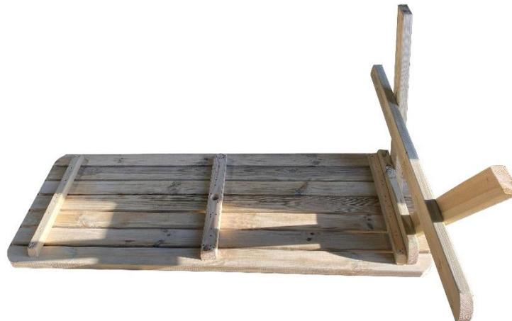
Place one of the table A-frames centrally against the fixing batten ensuring that the gap at the table edge is the same on both sides.
