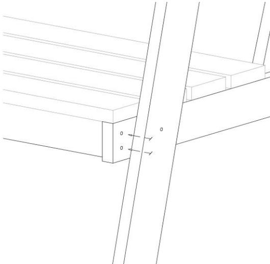
Align the seat panel flush with the front edge of the end frame as shown and secure in place using 2x 85mm screws. Repeat for the other leg frame.
