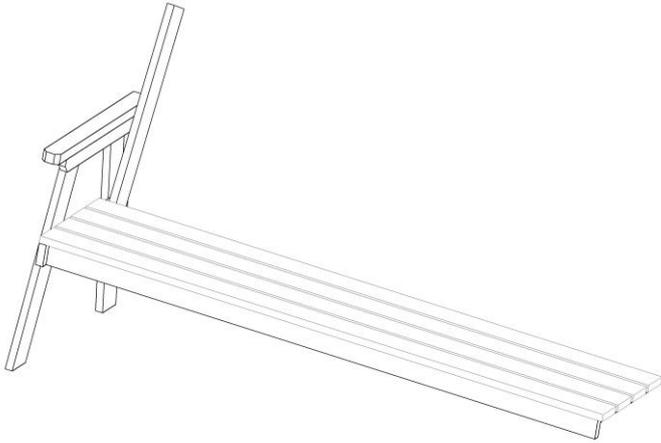
On a flat, level surface. Slot the seat panel into the leg frame as shown above.
