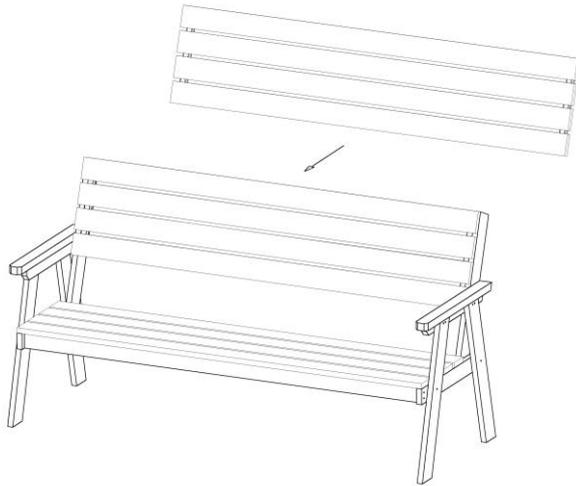
Place the backrest panel into position. (It is recommended to use an assistance for this step if possible).
