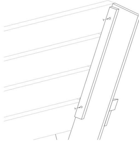
Secure in place using x2 coach screws.
