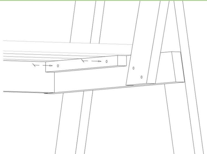
Working from underneath the seat panel use 2 coach screws to attach the seat panel to the leg frame and then repeat for the other side.
