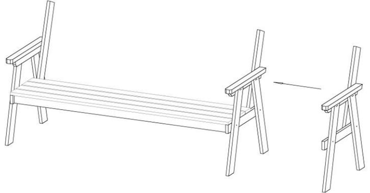
Now lift up the other side of the seat panel to place the other leg frame in place. (It is recommended to use an assistance for this step if possible).
